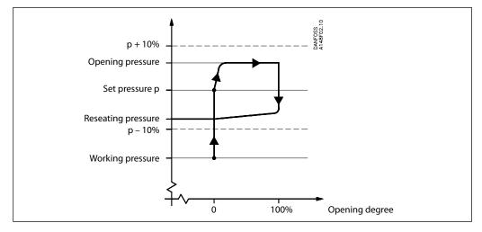
SFA is designed as a **standard safety relief valve** (DIN 3320), which is recommended for refrigeration plants. On a rise in pressure above the set pressure, the safety relief valve will initially start opening slightly, to minimise the outlet of
